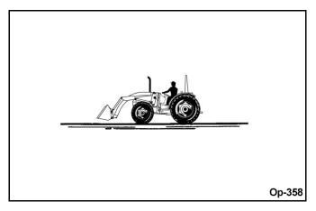
Use extreme care when operating loader on a slope, keep bucket as low as possible. This keeps center of gravity low and will provide maximum stability.
